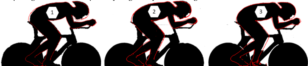
Figure 1. Geometric comparison using side contours of virtual geometry (red) and geometry during WT tests (black)
